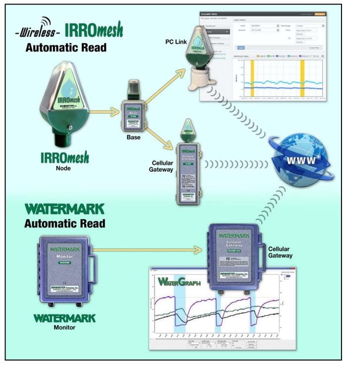
Monitoring soil moisture data from multiple sites or remote locations is now simpler with WATERMARK Remote Data Access equipment. Advances in communication technology provide cost effective and reliable methods of improving productivity and lowering operational costs by bringing the soil moisture
